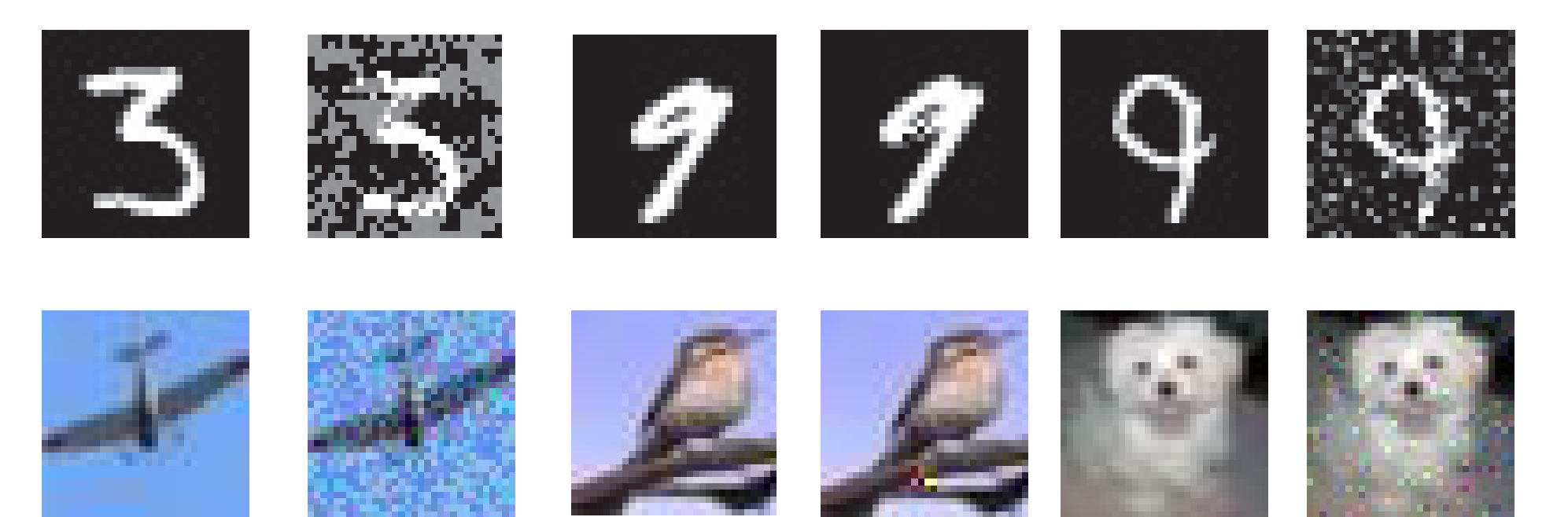
Fig. 3. The examples of original images and the three attacks' adversarial samples. The first row shows the images from MNIST while the images in second row are from CIFAR-10. Three adversarial attacks (FGSM, LSA, PSO) are used to perturb the original images. The three attacks use different modification patterns which cause the images are classified incorrectly.
